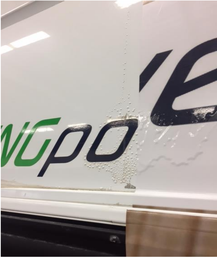
Attachment 3 – CNG Bus Kamloops Paint Blister
