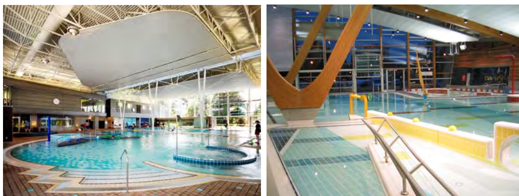
Above: Free-form leisure pool tanks with some lap/lane capacity have proven very popular and typically include seating opportunities, various water play features (sprays and jets in the pool, on the pool deck and suspended from the ceiling), easy entry (zero-depth beach or ramp), a lazy river, a vortex or bubble pit as well as water surface area that accommodates aquatic programs and lessons. The actual shape and configuration of a leisure pool is best designed with significant staff and stakeholder involvement to ensure it suits the actual needs of the specific facility. (Image 1: Chimo Aquatic Centre, Coquitlam, Image 2: West Vancouver Aquatic Centre)
