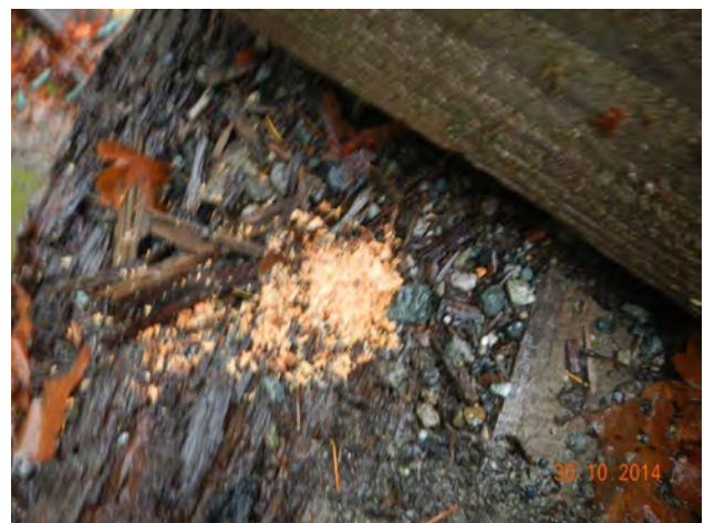
Drill sampling - shavings from top of log
