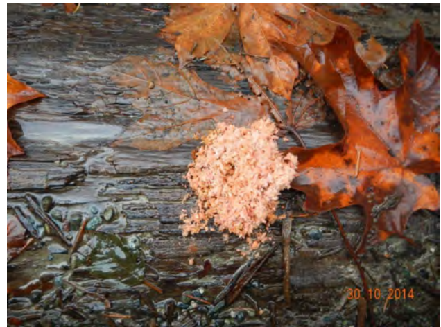
Drill sampling - shavings from side of log
