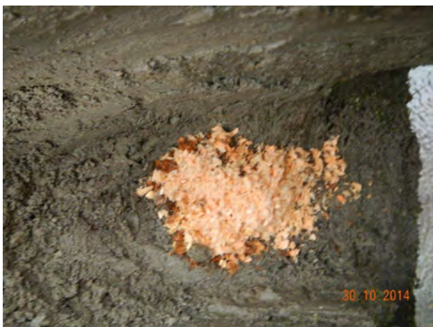
Drill sampling - shavings from top of log
