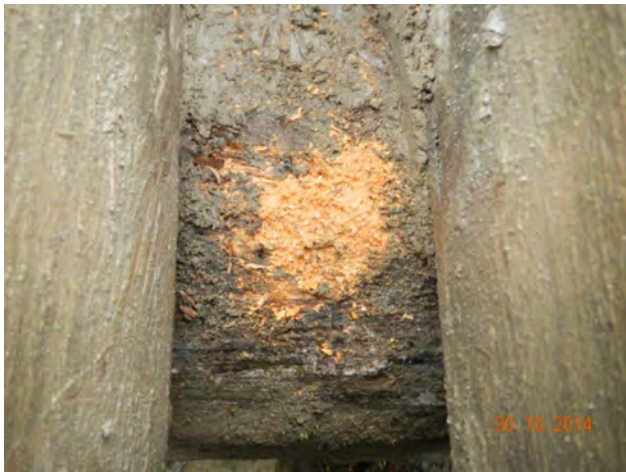
Drill sampling - shavings from top of log
