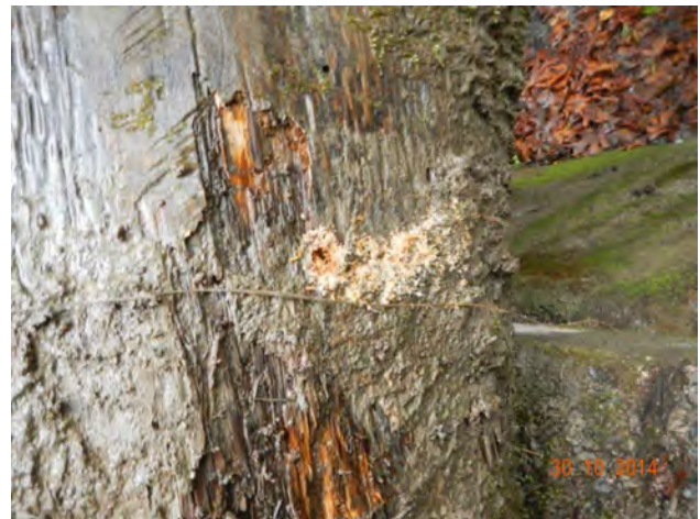
Drill sampling - shavings from side of log
