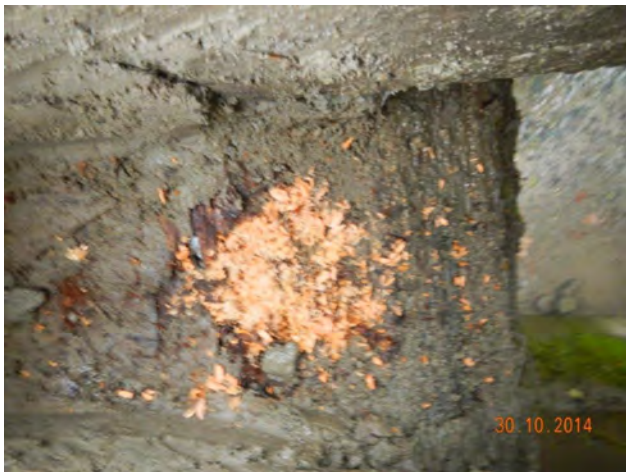
Drill sampling - shavings from top of log
