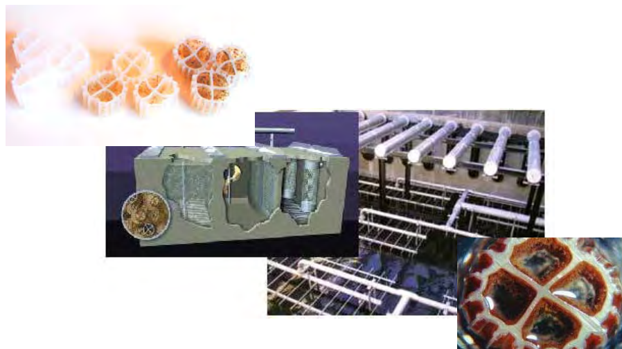
Figure 6 Moving Bed Biofilm Reactor
