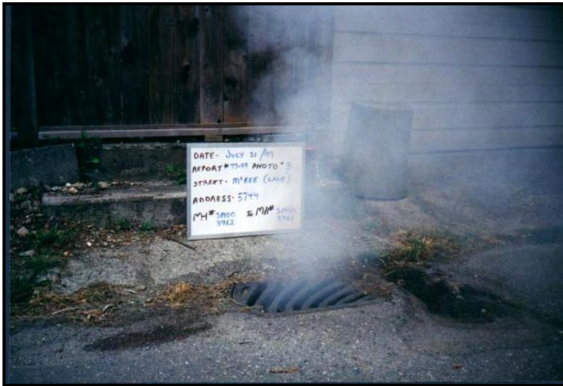
Figure 6. Vapour escaping from abandoned services
