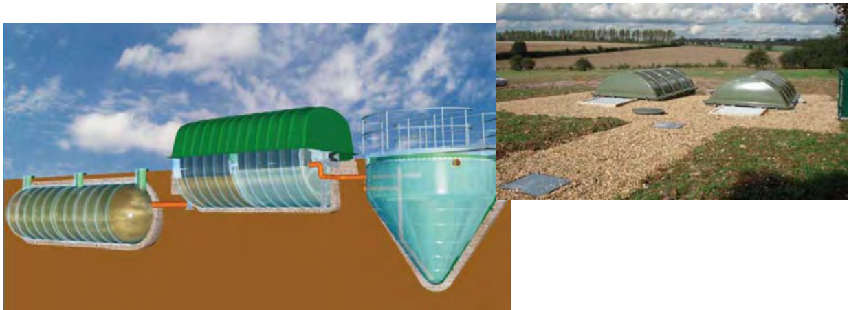
Figure 3 Rotating Biological Contactors
