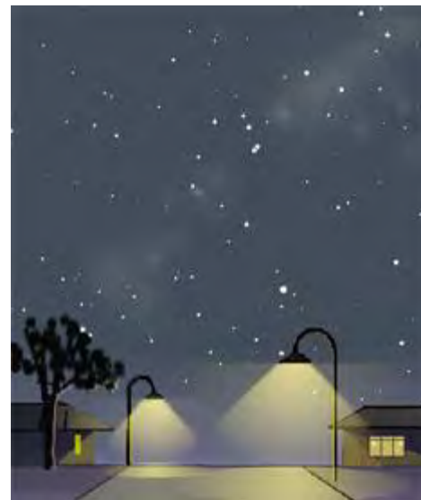
Full cut off light fixtures direct light below the horizontal plane reducing light pollution and protecting the night sky.
