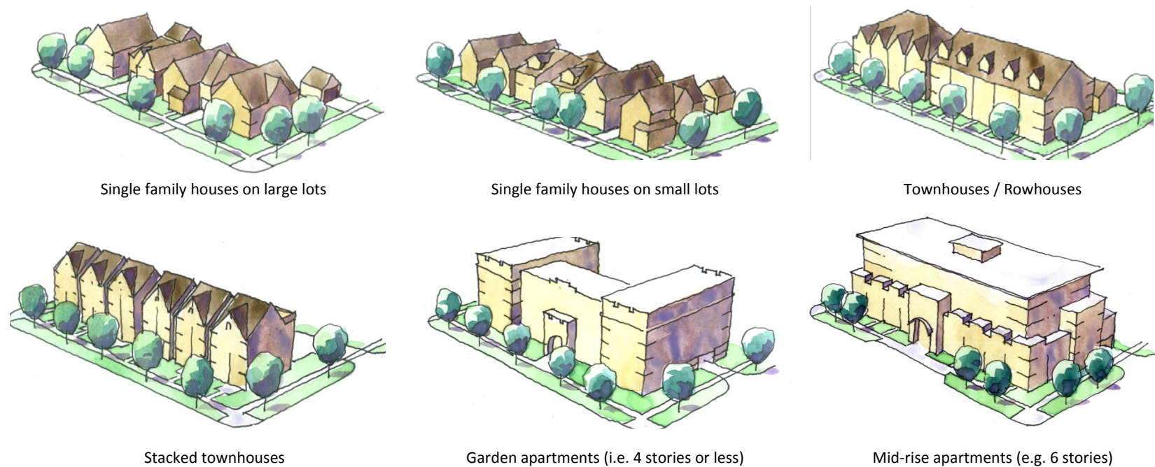
Figure 4 - Examples of housing typologies. A community's overall residential density accounts for all units, which usually include different housing typologies. While multi-family units help communities achieve densities that support walking and transit, single-family houses on small lots can also achieve this.
