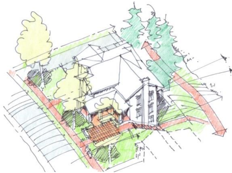
Illustration showing how topography or creative roofscape architecture can fit a third floor into the roof or as a walkout basement.
