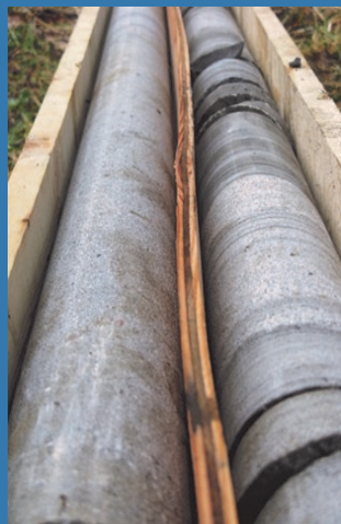
Rock Core from the Yellow Point Aquifer Observation Well
