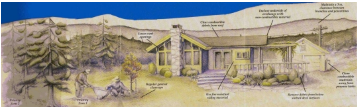
Diagram. FireSmart homes and properties feature fuel modification zones and fire-retardant construction.
